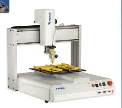
The model F4400N provides a generous working area of 15.75" x 15.75" (400 x 400mm). Fisnar robots interpolate in all axes for 3D dispensing of adhesives, silicones and UV Cure resins.
