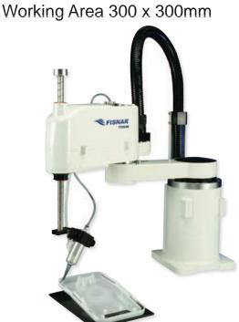
A 4 axes high-speed industrial SCARA robot ideal for high volume and large area dispensing applications requiring greater flexibility for automated manufacturing environments, including conveyors and work cells. Can also be used for pick & place applications.
