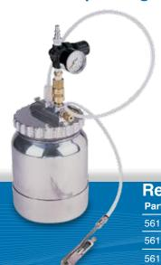
The needle valve pen simplifies the application of a low to medium viscosity fluid, which is not affected by contact with metal parts. Material is fed into the pen from a cartridge or reservoir. The finger control shut off instantly opens and closes the material flow. The pen is suitable for microdots, beading and potting operations.
