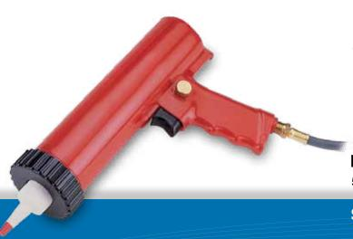
Dispense caulk and sealant materials. Connect the 580112C to a regulated air supply to dispense directly from the caulking tube. Most materials will dispense satisfactorily from 12 to 30 psi (0.80 – 2.0 bar). Do not exceed 60 psi (4 bar).
