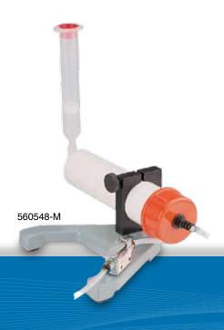
The model 560548-M loads a barrel directly from a 1/10 gallon caulking tube. The model 560022-M loads a barrel from a 12 ounce cartridge. The barrel loader is connected to an air regulator and set to a pressure suitable for the material but less than 65psi (4.48 bar). A switch on the side of the stand activates the airflow and is switched off when the material reaches the desired level. The barrel attachment assembly is threaded to accept luer lock barrels.
