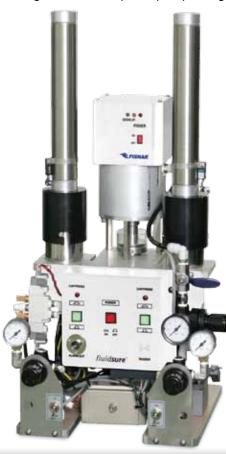
The EP1320C tandem cartridge pump is designed to easily transfer material for controlled dispensing via a high pressure valve. The suitable viscosity range is 10,000cps - 600,000cps. Rated at 15:1 the system provides a maximum of 995 psi regulated material pressure. The A & B cartridge management automatically switches from either A to B or B to A when the cartridge is exhausted. Cartridges are contained in metal jacketed cylinders.
