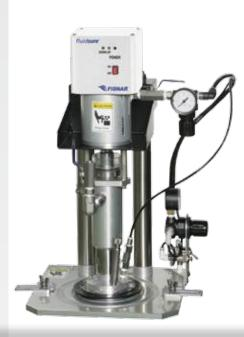
The EP1301N is designed for a 1kg (1qt) can of medium to high viscosity fluid. The EP1303N is configured for a 3kg (1 gallon) can of similar viscosity. Both systems are rated at 15:1 and provide a maximum of 996psi regulated material pressure.
