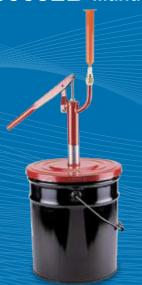
Trying to extract material from large pails can be a daunting project. The pail pump is a simple solution. Suitable only for 5-gallon straight-walled pails containing fluids, such as grease, paste, etc. The hand lever pumps the fluid to bottom-fill 2.5, 6, 8 or 12oz cartridges together with luer lock barrels from 3cc up to 55cc.
